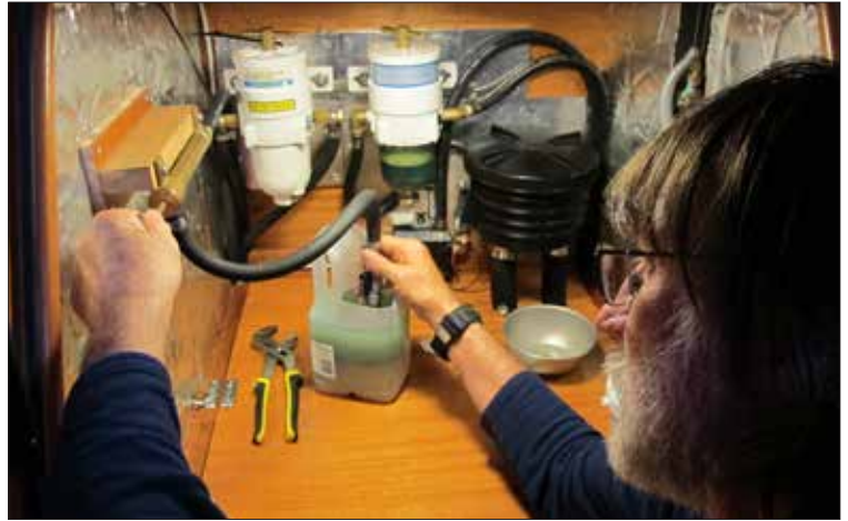
Left —Before any fuel goes in his tanks, the author takes a small sample to see if it is crystal clear. Right —With his manual fuel-tank-sampling pump, the author takes samples at the beginning of every boating season, periodically during the season, and at every refueling.
