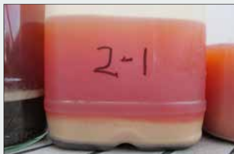
Water-saturated diesel taken on board in the U.K. Left to right —The three samples represent the water that has settled out at the base of the tank immediately after refueling, 24 hours later (2-1), and then another 24 hours after that (3-1). The rate of water dropout decreased but nevertheless continued for weeks.
