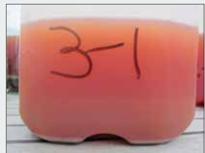
Water-saturated diesel taken on board in the U.K. Left to right —The three samples represent the water that has settled out at the base of the tank immediately after refueling, 24 hours later (2-1), and then another 24 hours after that (3-1). The rate of water dropout decreased but nevertheless continued for weeks.
