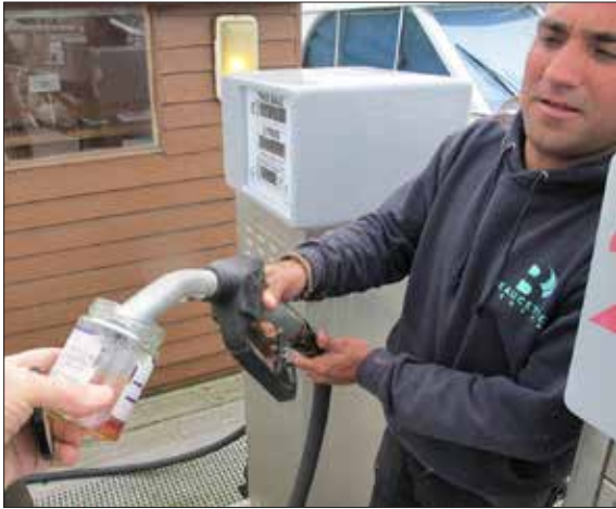
Left —Before any fuel goes in his tanks, the author takes a small sample to see if it is crystal clear. Right —With his manual fuel-tank-sampling pump, the author takes samples at the beginning of every boating season, periodically during the season, and at every refueling.
