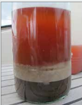
Water-saturated diesel taken on board in the U.K. Left to right —The three samples represent the water that has settled out at the base of the tank immediately after refueling, 24 hours later (2-1), and then another 24 hours after that (3-1). The rate of water dropout decreased but nevertheless continued for weeks.
