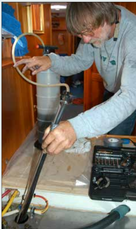
In an unsuccessful attempt to pull contaminated fuel from the bottom of his tank, the author employed a suction tube duct-taped to a stick fed through a 2" (51mm) hole. That access proved too small to properly clean the tank.
