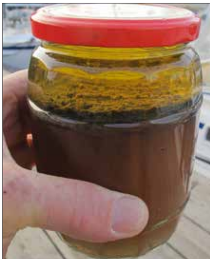
Above —This sample of the fuel taken on board at a high-end marina in Sweden shows a likely combination of bacterial fouling and gunk broken loose from the marina's fuel tank by the biodiesel's solvent properties. Right —A series of samples illustrates the progression of serious saltwater contamination from the base of a tank upward. The saltwater contamination occurred in heavy weather through a poorly sited tank vent.
