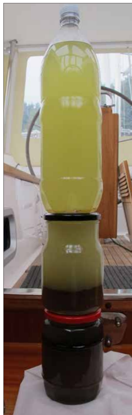
Above —This sample of the fuel taken on board at a high-end marina in Sweden shows a likely combination of bacterial fouling and gunk broken loose from the marina's fuel tank by the biodiesel's solvent properties. Right —A series of samples illustrates the progression of serious saltwater contamination from the base of a tank upward. The saltwater contamination occurred in heavy weather through a poorly sited tank vent.
