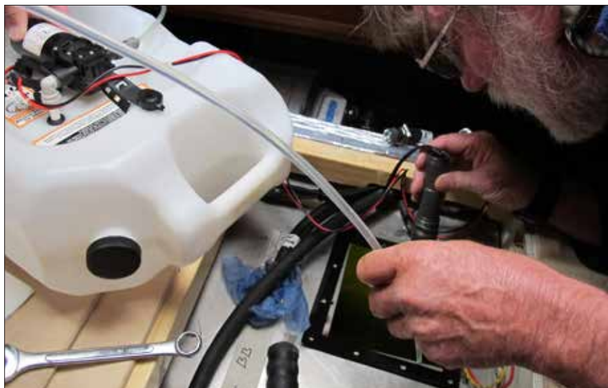
In the author's initial attempt to pump down a contaminated fuel tank, a lightweight oil-change pump proved totally inadequate to the task.
